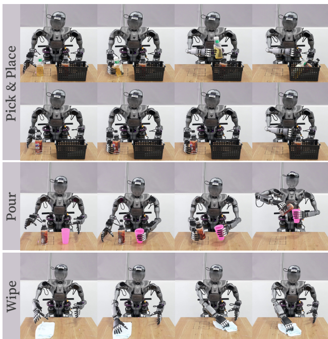
Fig. 5: Trajectories of our three tasks in the training scene, including Pick&Place, Pour, and Wipe. We carefully select daily tasks so that they are useful across scenes.
