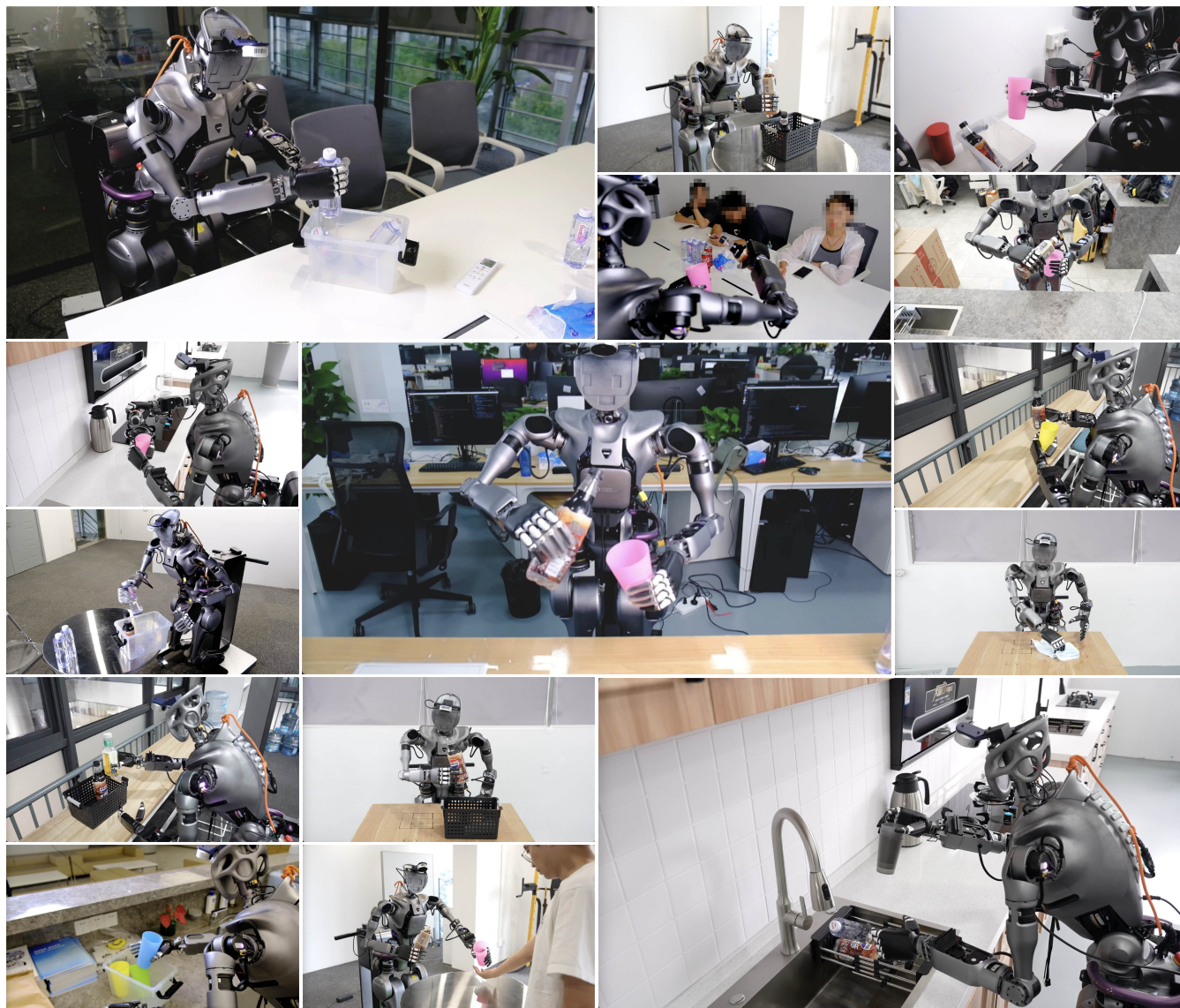
Fig. 1: Humanoid manipulation in diverse unseen scenarios. With only data collected from a single scene, our Improved 3D Diffusion Policy (iDP3) enables a full-sized humanoid robot to perform practical skills in diverse real-world environments. The scenes are not cherry-picked. Videos are available on our website.
